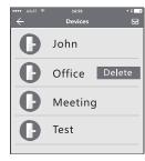
To delete the lock, find the name and click to find the delete button, you can delete the lock in the APP. Also you can long press the reset button on the rear side of front panel, so the other user can add this lock as new device.
